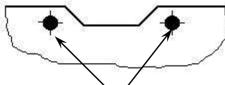
Nails Ø 3 x 30 / Self-drilling screws ø 4,8 x 25 mm
